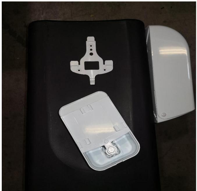
11) Transfer the drill holes from the back of the #3 Dispenser to #1 trash can and drill them as well with the 5mm drill bit. Then rivet them with #9 rivet. Repeat this on the opposite side of the #1 trash can.
