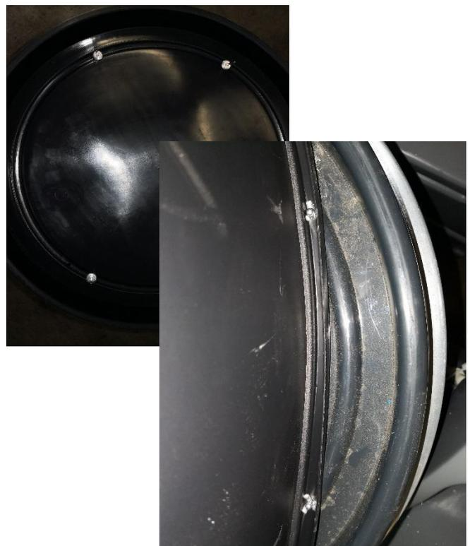
15) Put the lid of the barrel back on, fix it with the clamping ring.
