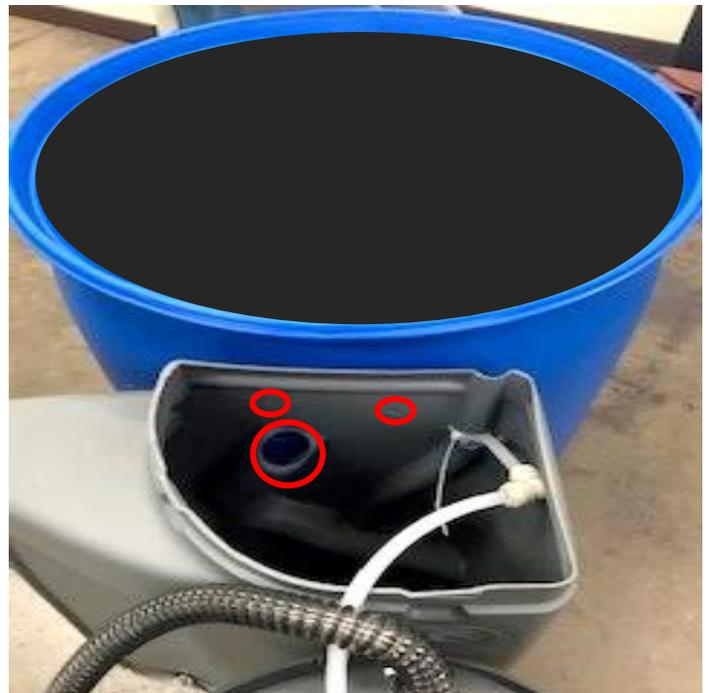
3) Drill the 5mm holes with the 5mm drill through the barrel.
